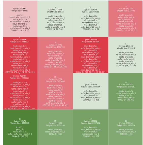
Fig. 5. Mapping information ResNet50 mapped in a 16 tile system with a 4096 KB Tile Weight Capacity.
